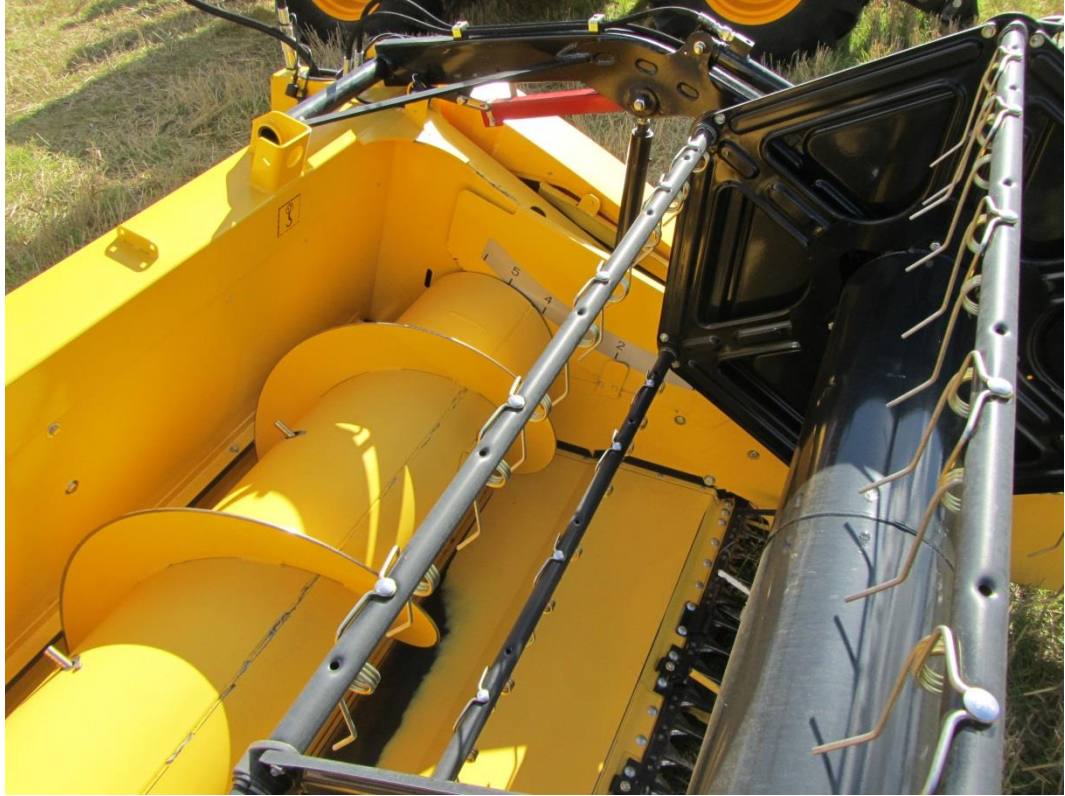
Picture 5. Header with adjustable length – the bottom can slide forwards. Photo: Henning Sjørøsløv Lyngvig
