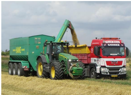
Picture 28-1 and 28-2. Auger-wagon delivering grain to a lorry or a tractor with an on-road wagon. Photos: Henning Sjørslev Lyngvig
