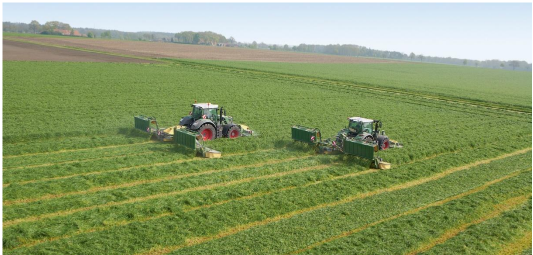
Picture 16. Cutting grass with a disc mower. Belt conveyers can be lowered to collect in swaths, if required. Photo: Krone
