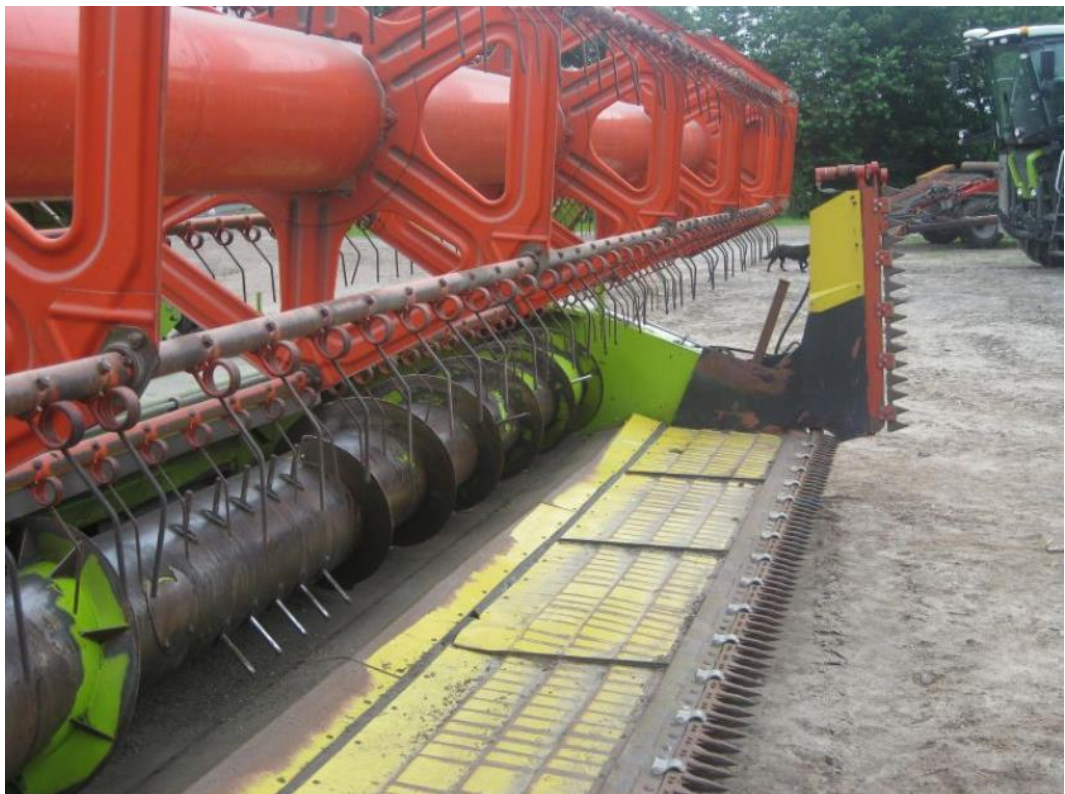
Picture 4. Unit for making the header longer with side knives included. Photo: Mosegaarden
