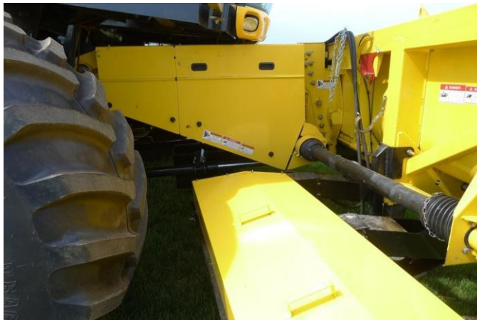
Picture 14-1 and 14-2. The stems are blown to a belt conveyor (under the yellow cover behind the header), and placed between the wheels of the combine. Photo: Cornrower / Henning Sjørsløv Lyngvig
