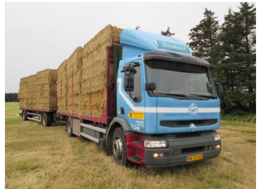
Picture 31-1 & 31-2. Bale size and density decides how many tonnes per load are transported. Photos: Mosegaarden
