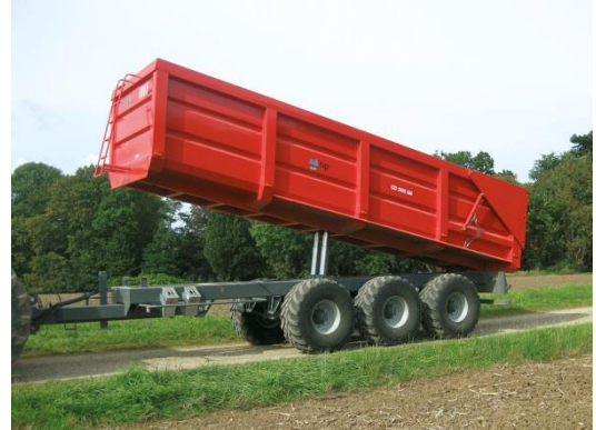
Picture 27-1 and 27-2. Two examples of off-road wagons for grain and rape. Photos: Baastруп and MI.
