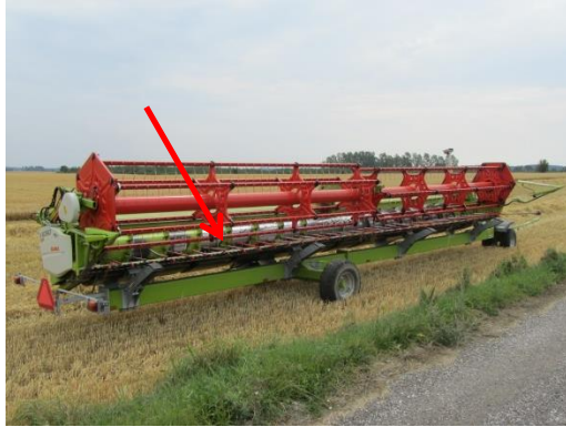
Picture 2. Standard header with an auger. Photo: Henning Sjørslev Lyngvig
