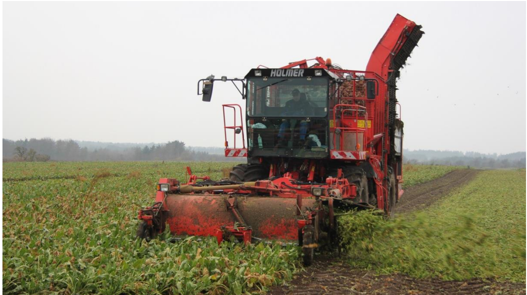
Picture 7. Large self-propelled beet lifter with beet topper in front. Photo: Søren Ugilt Larsen
