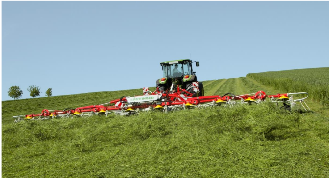
Picture 17. Grass dries faster if dispersed by a tedder. Photo: Pöttinger
