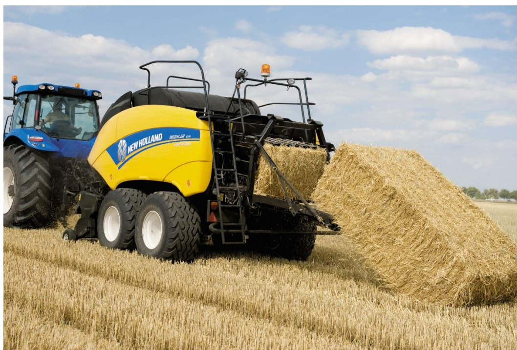
Picture 22. Baling straw from grain. This type of bales is approximately 80 x 120 x 220 cm. Photo: CNH
