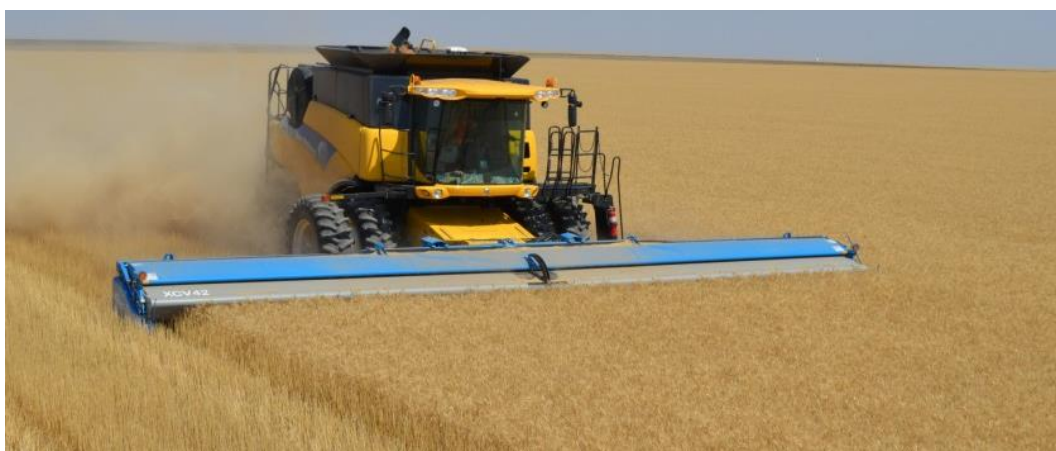
Picture 32. Using a stripper header the straw is left on the field. Photo: Shelbourne Reynolds
