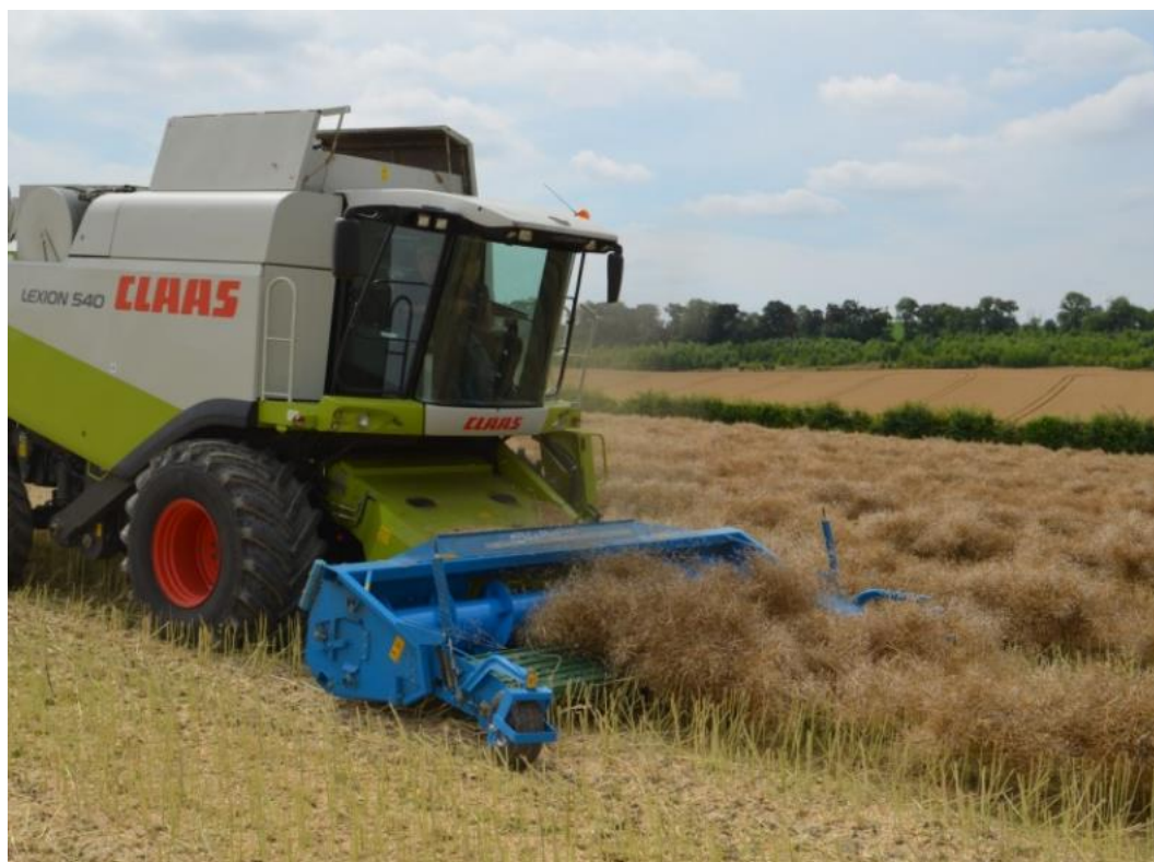
Picture 6. Harvesting rape with a pick-up header. Photo: Shelbourne Reynolds
