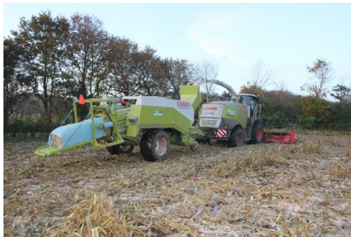
Picture 24-1 & 24-2. Baling and wrapping maize straw in plastic. The job is done in two steps.
