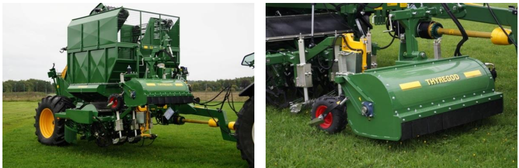
Picture 8-1 and 8-2. Tractor-propelled beet lifter with topper. Photo: Thyregod
